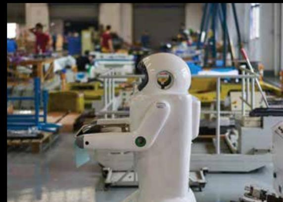
**Above:** the Shangpin Home Collection factory where the use of robots to cut and drill wooden planks improved productivity by 40 per cent.
